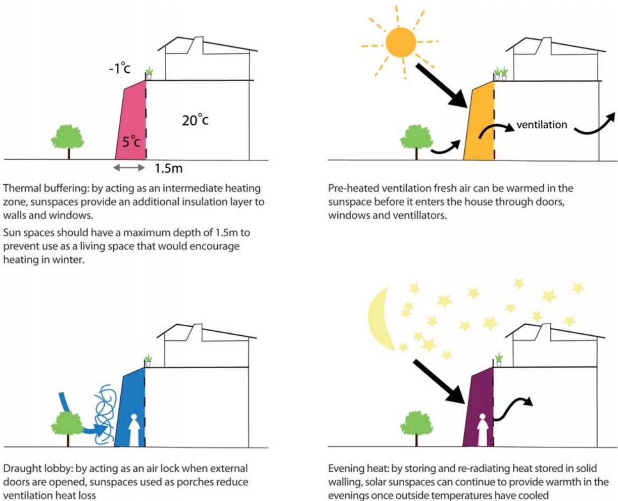
Thermal buffering: by acting as an intermediate heating zone, sunspaces provide an additional insulation layer to walls and windows.
