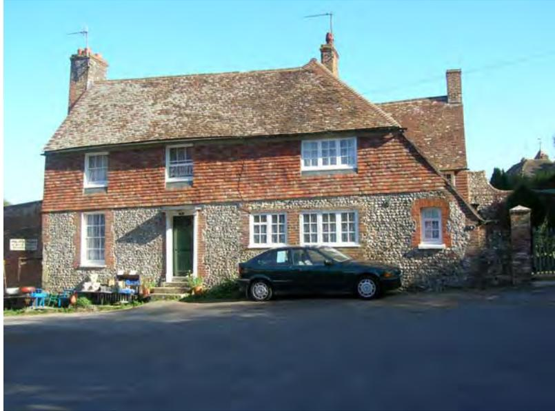
Hand made red tiled first floor and roof, field flint ground floor with red brick detail around windows at 4 and 5 The Street
