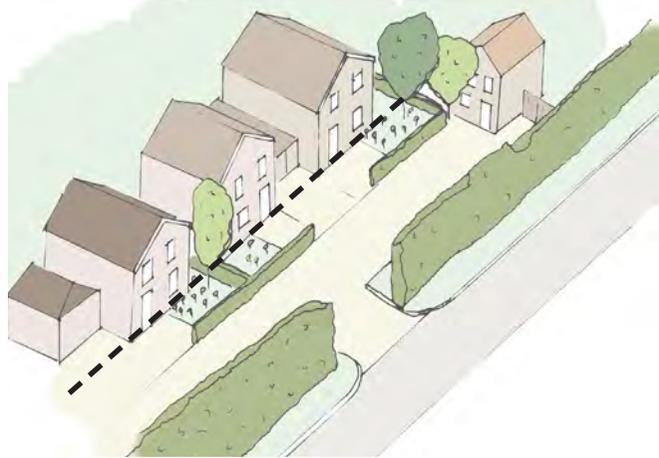
Figure 313. Diagram showing a consistent building line.
