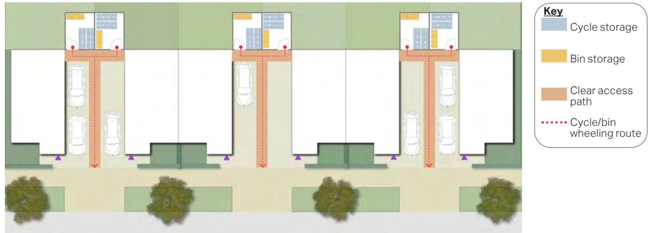
Figure 338. Diagram showing combined cycle and bin storage location and access from the rear.
