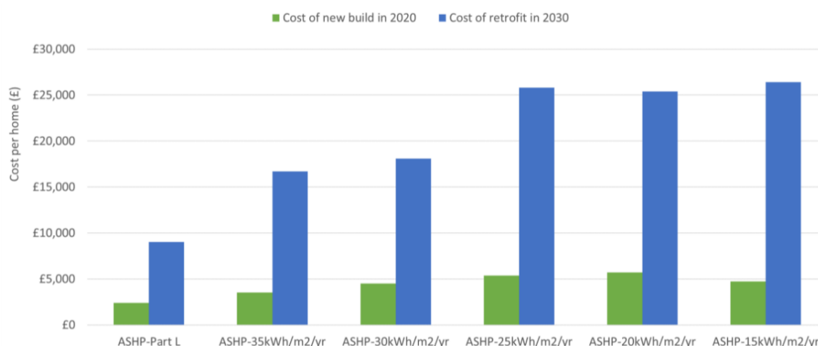
Figure 9: Graph showing the additional costs of installing ASHP and meeting space heating standards in a new semi-detached house compared to retrofitting these after construction.
